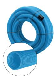
Unperforated corrugated PP drainage pipe; colour blue; ring stiffness larger than or equal to 10 kN/m² ("SN 10"); in conformity with DIN 1187 and DIN 4262-1.
