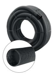
Totally perforated corrugated PE pipe; colour black with yellow coloured stripe; ring stiffness class SN 8; total perforation area larger than or equal to 50 cm²/m; 1.2 mm perforation width.
